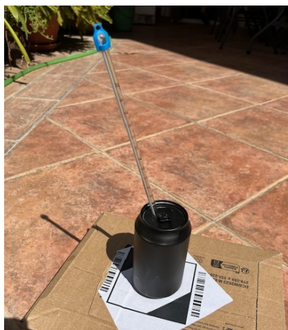
Figure 1: A water filled can with a lid and thermometer, sitting on an insulated base in the sunshine.
